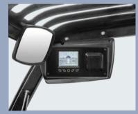
Large screen display, the instrument panel adopts njection molding design, sturdy and durable
