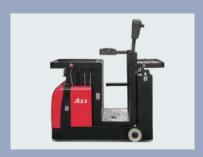
The guardrails are equipped with detection switches. The order picker cannot work until the guardrails are put down
