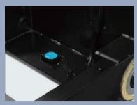
The tilt sensor prevents the vehicle from tipping due to excessive slope and ensures operator safety
