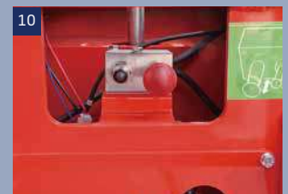
Manual release valve: When the machine can not move, you can push the machine after pressing this valve
