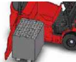
Battery side removed by forks (Opt.)
