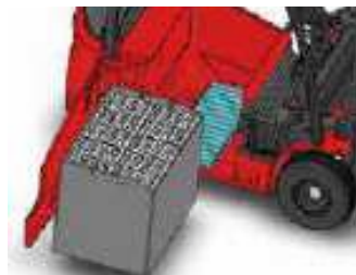
Battery side roll out by roller (Opt.)
